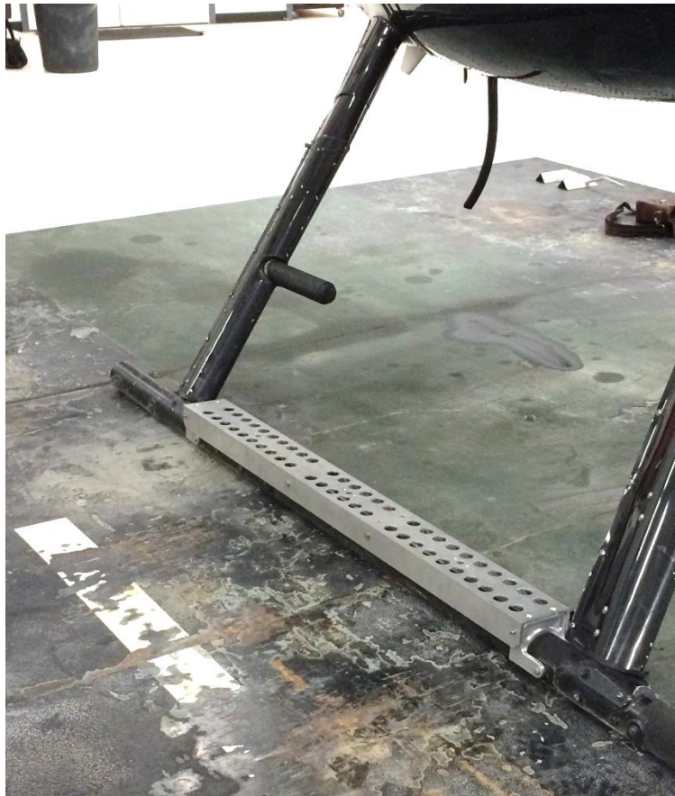
Figure 1. Skid Step Assembly Installed on MD 369FF Model Rotorcraft
